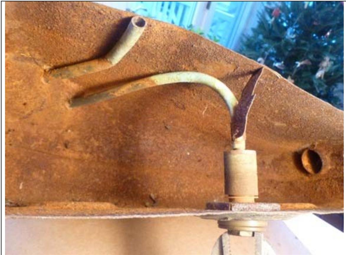
This long view shows the opening at the far end where fuel from the filler neck enters. In the foreground is the filter and tube in their correct positions. At the top is the tube that allows displaced air to return to the filler neck as the tank as fuel level rises during fillups. When this line is plugged, you will have difficulty filling rapidly.
