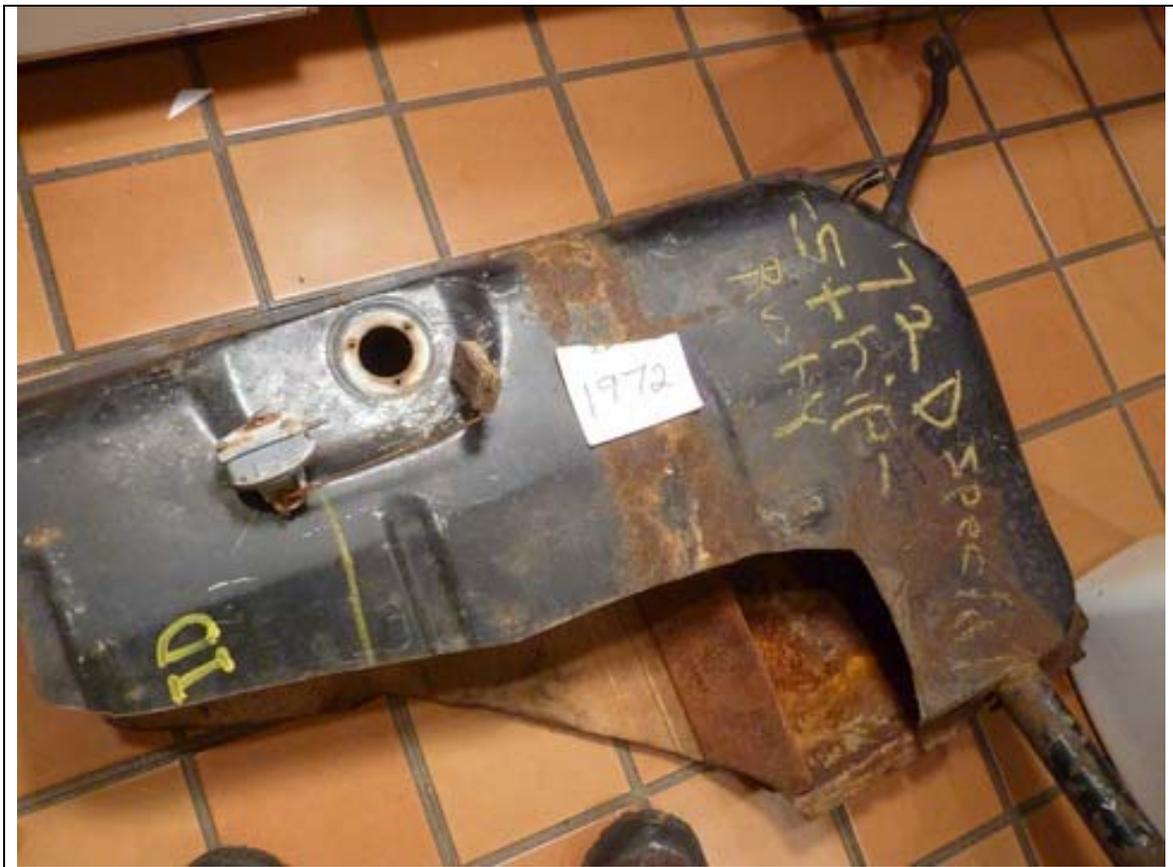
Shown here is a tank from a carburetor car. There is one fuel outlet and one air return to the filler neck at the upper right. To the lower right is the filler neck. Note the fuel sender laying across the top near its opening. You can also see the inside, where a sloped baffle keeps a supply of fuel at the filter/pickup area under most conditions.
