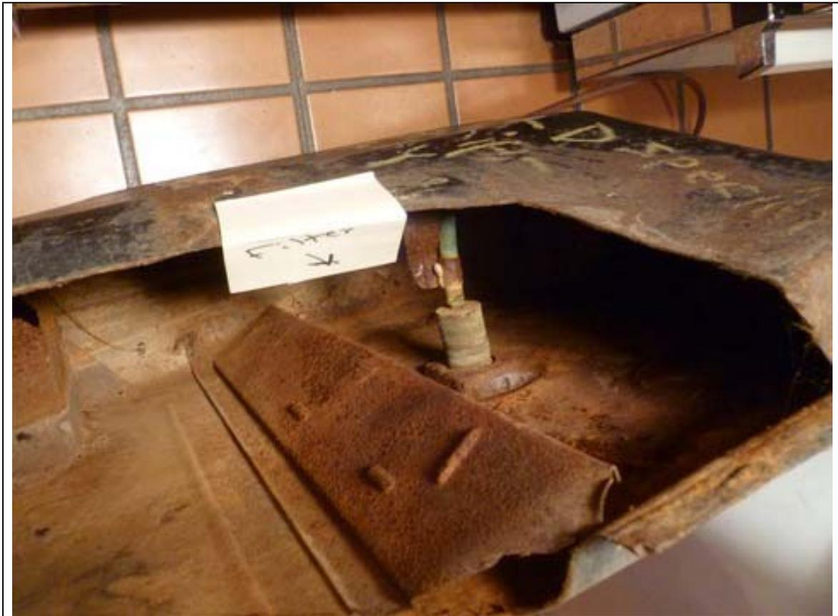
A side long view shows how the metal tube that carries the nylon fuel line straight down to the filter. Just above the filter is a flat piece of metal that is spot welded to the top of the tank and the tube. To the left is a partial view of the fuel sending unit baffle. Going straight across the bottom is the fuel retaining baffle. This is in effect a reserve.
