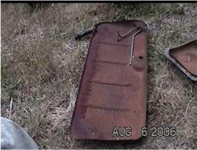
This shot of the interior of an inverted tank from a carbureted car shows the layout of the tubes as shown from the bottom looking up. The pickup tube is pointing upward and is held in place by a spot welded piece of sheet metal near its end. To its right is the filler air return tube. Just to its right is the opening for the fuel sending unit. The filler neck points off to the upper left.
